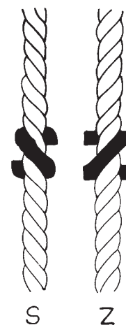
Fig. 2.12. An s- and an z-spun thread (drawing: Annika Jeppsson).
