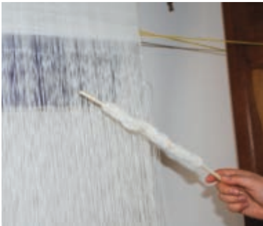
Fig. 4.3.6. (right) Wooden sword used as a weft beater (photo: CTR).
