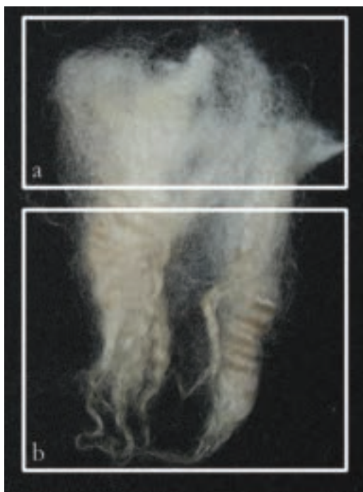
Fig. 2.7. Wool fibres (a) underwool (b) hair (photo: CTR).
