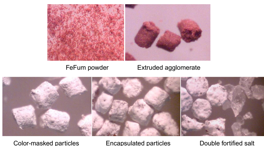
FIGURE 38.3 Evolution of ferrous fumarate premix during the DFS preparation process (digital microscopic images taken under normal room light) (Li, 2009).
