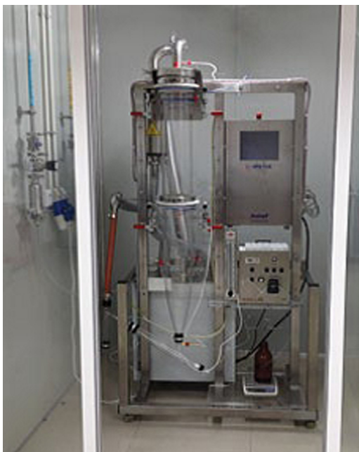
FIGURE 5.2 Spray dryer from ProCepT.
