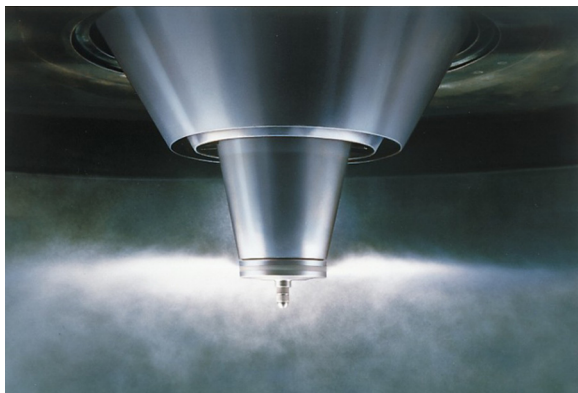
FIGURE 5.12 Rotary atomizer designs. Courtesy of GEA Process Engineering.
