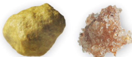
FIGURE 9.4 Product samples produced by agglomeration using high-shear processing (left) and fluidized bed technology (right).
