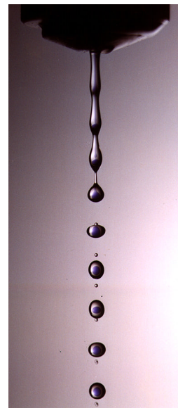
FIGURE 5.5 Stream of fluid breaks up into smaller packets.
