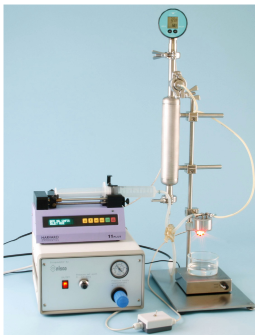
FIGURE 10.4 Coaxial air flow droplet generation. Courtesy of Nisco Engineering, Zürich, Switzerland, www.nisco.ch .
