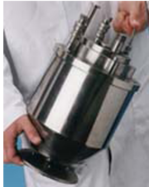
FIGURE 5.13 Rotary atomizer designs. Courtesy of Drytec Contract Processing.
