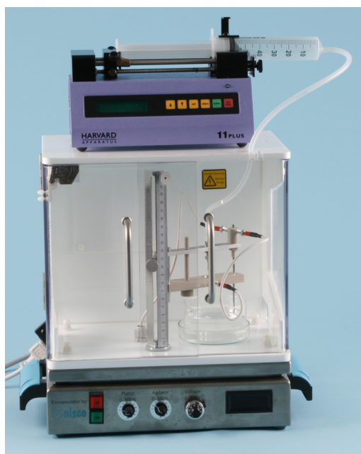
FIGURE 10.3 Nisco Var V1, electrostatically driven jet breakup. Courtesy of Nisco Engineering, Zürich, Switzerland, www.nisco.ch .
