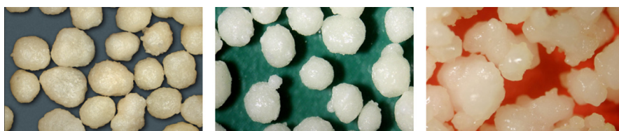
FIGURE 9.27 Formulation of vitamins. Granules produced by encapsulation in spouted bed: lavender oil (left), orange oil (middle), PUFA (right).
