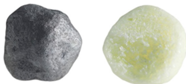
FIGURE 9.2 Product samples produced using spheronization of a wet agglomerate (left) and an extrudate (right).
