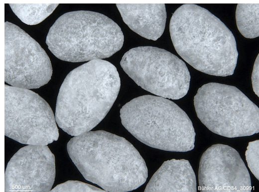
FIGURE 8.2 Samples of the extruded pellets with encapsulated flavor oils.
