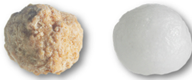
FIGURE 9.6 Product samples produced by spray granulation from suspension (left) and solution (right) using fluidized bed technology.
