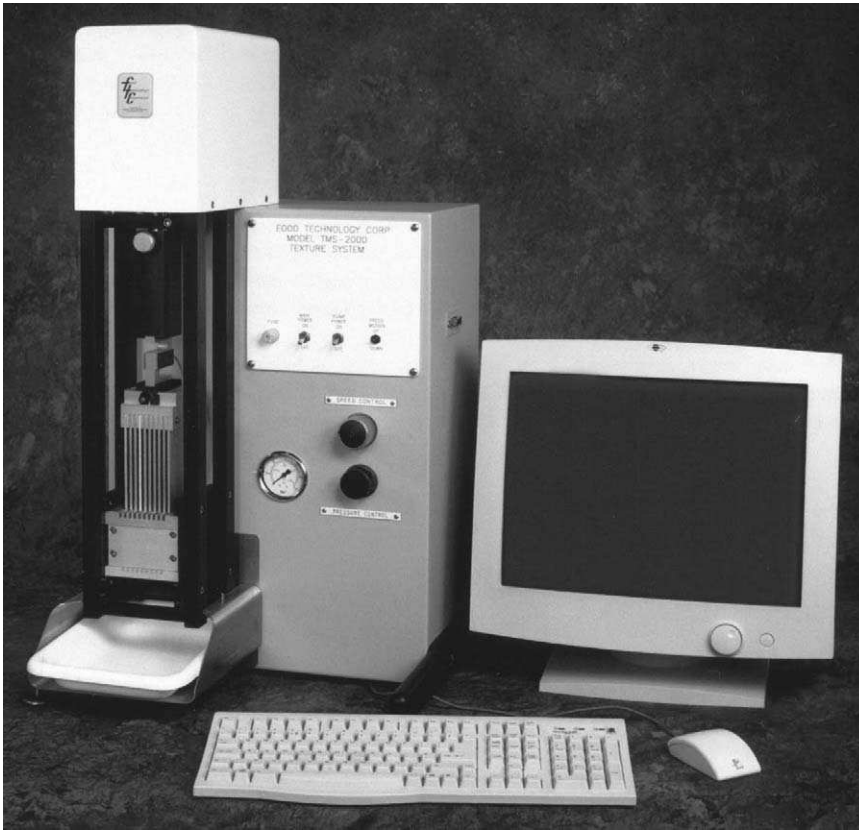
Figure 5.5 The Food Technology Corporation Texture Press (‘Kramer Shear Press’) Model TMS-2000. (Courtesy of Food Technology Corporation.)
