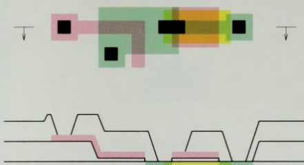
(e) Placing contact cuts.
