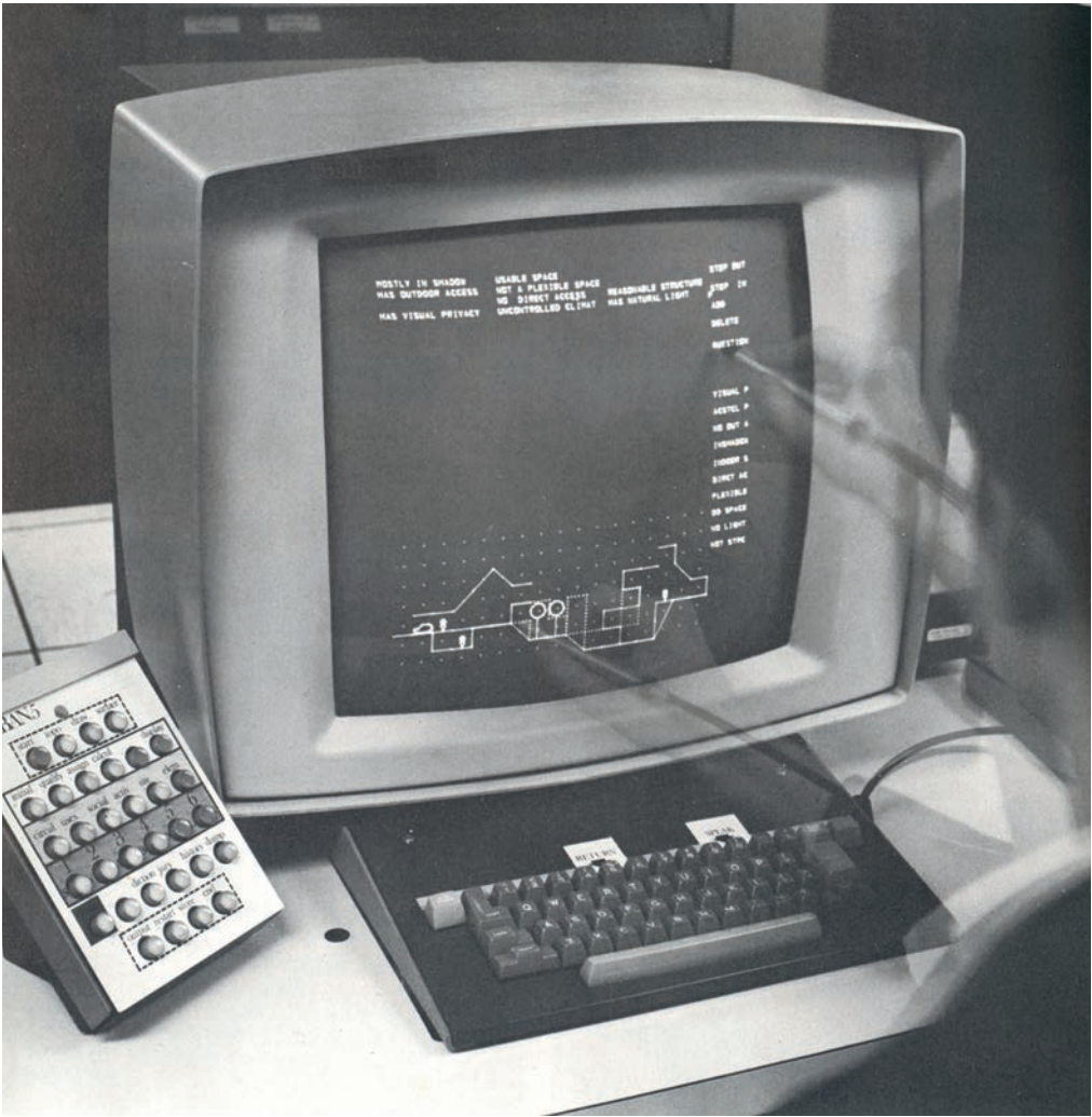
Architecture Machine Group, Interface for URBAN 5, with an IBM 2250, model 1 monitor, and scope connected to an IBM system 360/67, 1968.
