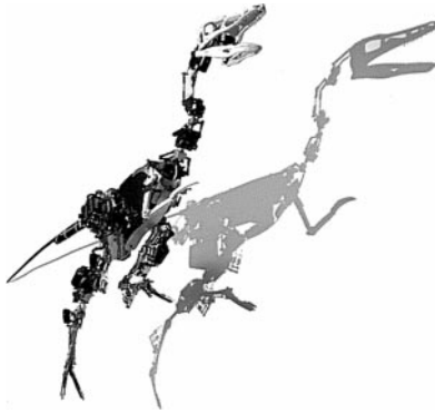
Figure 16.2 A special walking robot being designed and built by Peter Dilworth at the MIT Leg Lab. The robot is modeled after the dinosaur Troodon. It has legs with many degrees of freedom. At some point it should be able to stand up, walk, run, walk, and sit down again with smooth transitions. It will have its power supply and controller on board (reprinted with permission).
