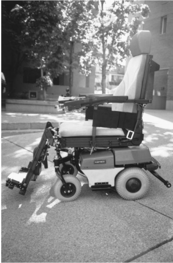
Figure 18.5 A semiautonomous wheelchair robot developed by Applied AI Systems in Ottawa, Canada (reprinted with permission).
